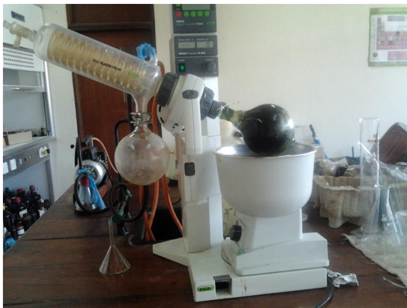
Figure 3. 1: The rotary evaporator unit
