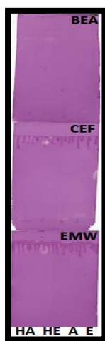
Figure 4.2: Chromatograms of S. monteiroae leaves after pre-treatment with hexane (HA=hexane for acetone and HE=hexane for ethanol) and then extracted with acetone (A) and ethanol (E).
