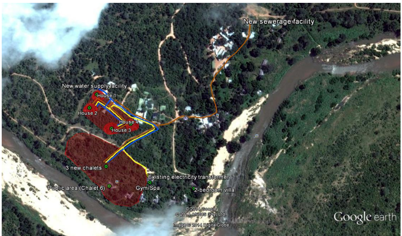
Figure 5: Potential electricity (yellow), water (blue) and sewerage (brown) utility routes which link to the developmental sites (Source: Google Earth 2014).
