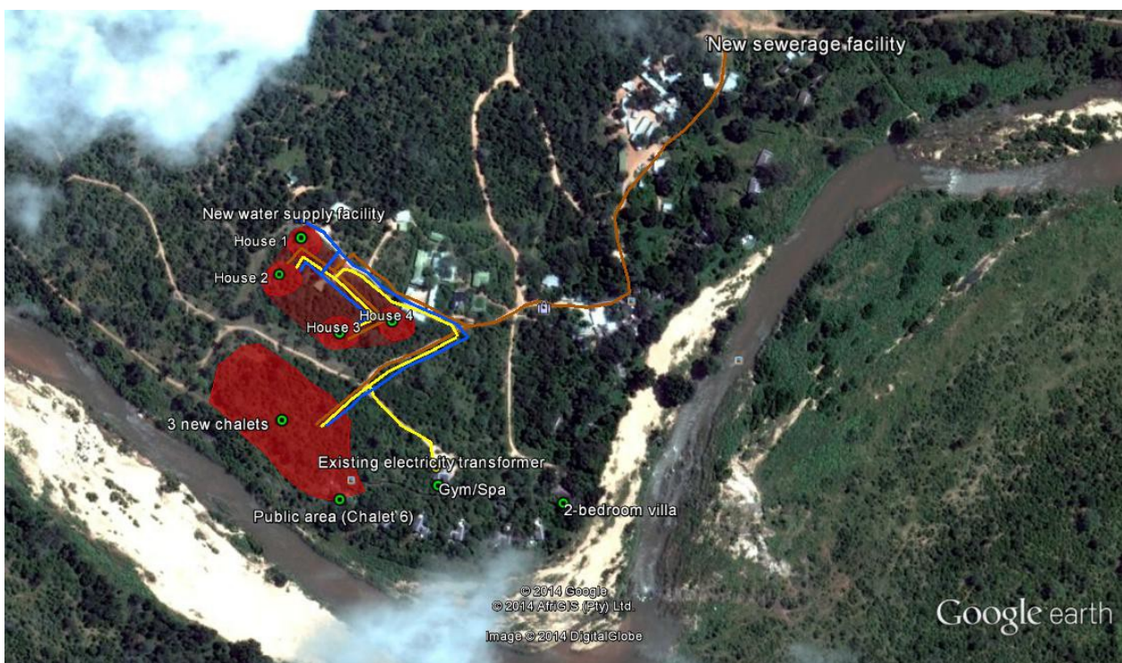
Figure 5: Potential electricity (yellow), water (blue) and sewage (brown) utility routes which link to the developmental sites (Source: Google Earth 2014).
