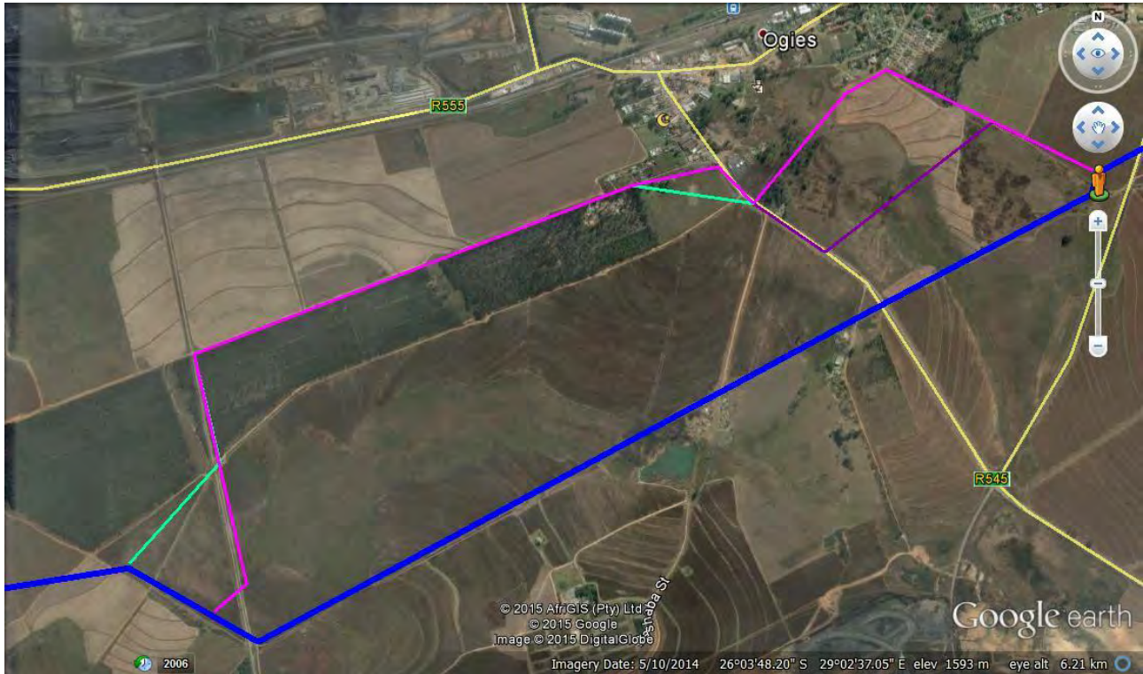
Figure 2- Map of the power line route alternatives showing the human land use in the area. (Map-Wildskies).
