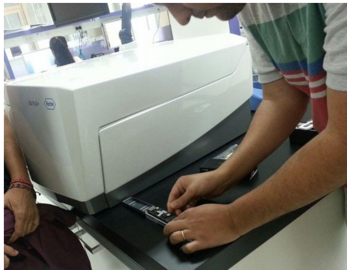
DNA sequencers timeline: on the left, an old Roche GS FLX+, on the right into the researcher hands, the Minlon. Invisible on this photo, a couple meters on the back of the photographer, 2 Illumina.
