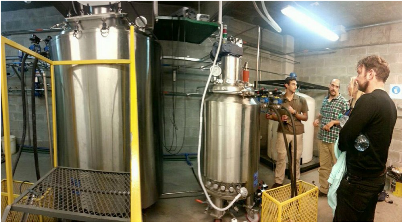
From left to right: Paul, Pablo, Tamra and Markku, in a partial panoramic view of the main 200 and 1000 l fermentors, filled to the brim with sensors and actuators.
