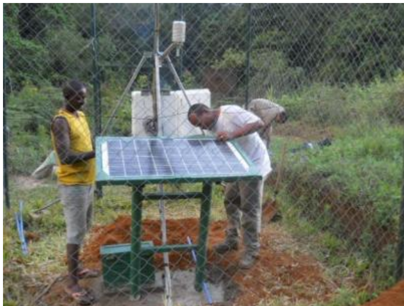
Figure 16. TEAM staff mounting a locking system for the solar panel at the climate station.
