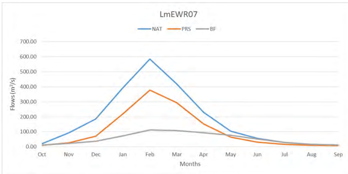
FIGURE I.11: HYDROGRAPHS FOR TRIBUTARIES AND MAINSTEM IN RISK REGION 11
