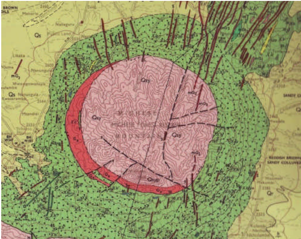
Figure 8. Portion of geology map covering Mt Mchese (1:100,000 sheet). Qsy = quartz-syenite; QsyP = quartz-syenite-porphyrity; Ga = granite; Xh = gneiss; mSy, S, D = dykes (syenite, dolerite).
