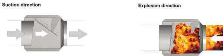
FIGURE 10: ILLUSTRATION OF THE FIRE CONTROL SYSTEM WITH A BACK-PRESSURE FLAP VALVE. SOURCE: ENVIROX, 2020
