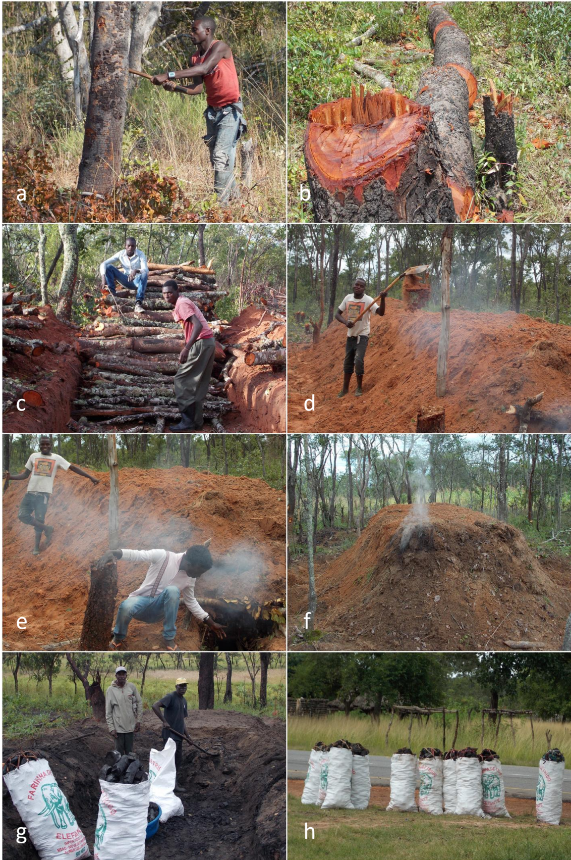
Figure 19: Observed charcoal production: (a) tree felling, (b) cutting stems into logs, (c) construction of the kiln, (d) kiln insulation with grasses, fresh leaves and earth, (e) ignition and combustion control, (f) carbonization, (g) sorting and packing of charcoal, (h) sale of charcoal along the roadside.
