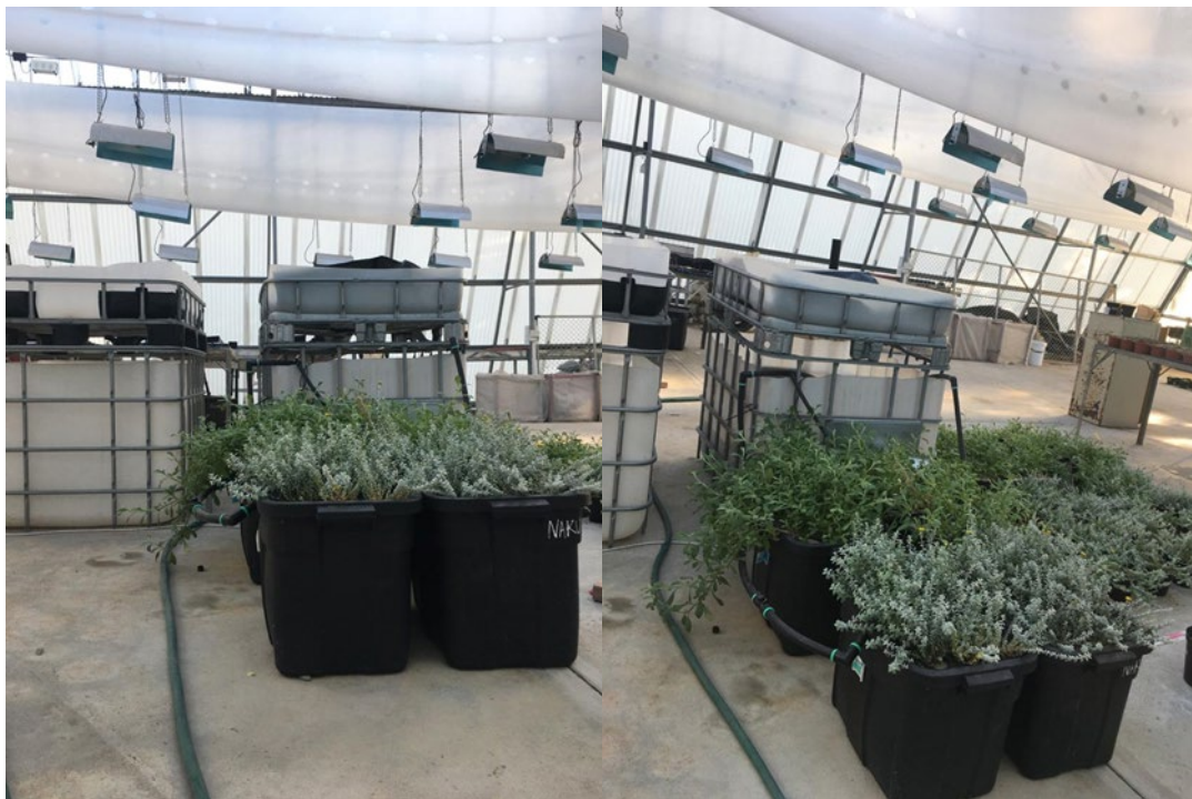
Figure 3.1: Experimental setup of aquaponic system with two 400L of fish tanks
