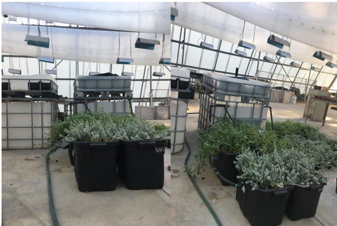
Figure 4.1: Experimental setup of aquaponic system with two 400L of fish tanks
