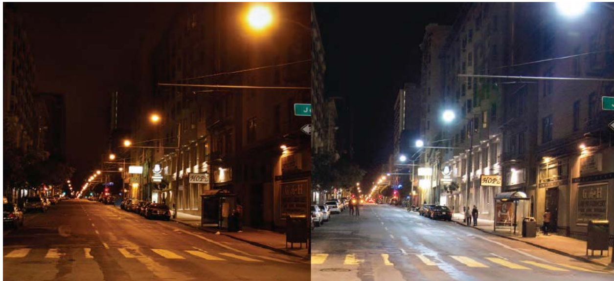
Figure 18. A comparison between lighting sources; HPS sources (left) and LED (right) (Bilsten et al. 2013).
