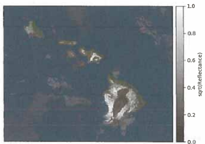
Figure 7. MODIS MYD09A1 RGB composite imagery for the month of 2014 May. [ R = band 1 (645 nm), G = band 4 (555 nm) and B = band 3 (469 nm)] Each band fluctuates between 0 and 1.
