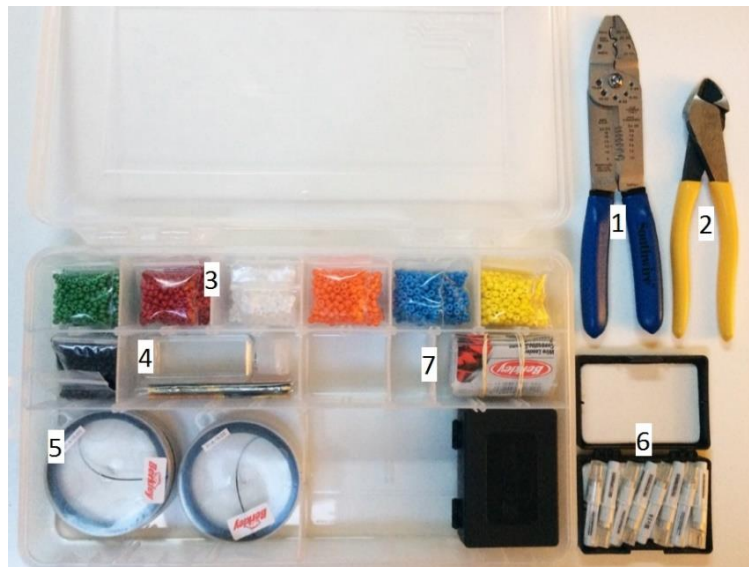
Figure. 10: Complete bead kit. 1: Crimp / Final Cutter tool; 2: Cable Cutters; 3: Seven different types of
