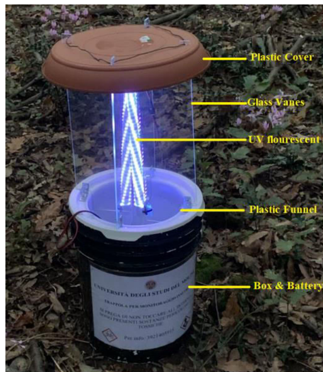
Figure 12. Partial View of the light trap used and description of its various components.
