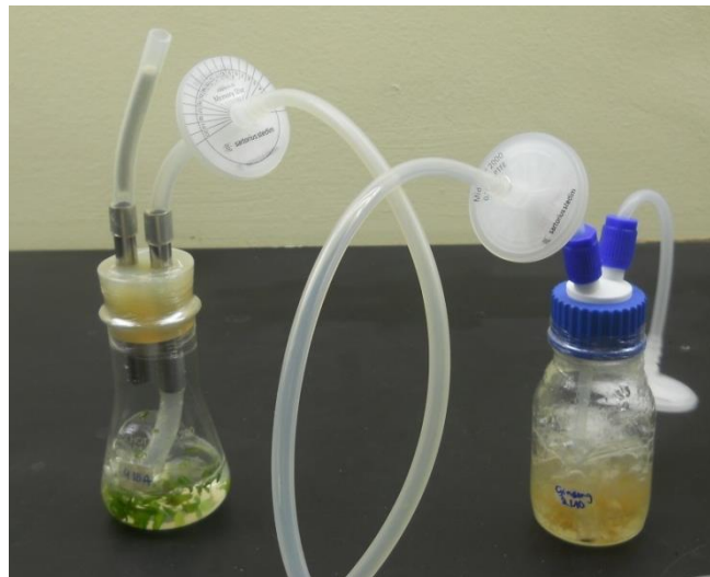
Figure 36: Small bioreactor made of an Erlenmeyer and a Duran bottle
