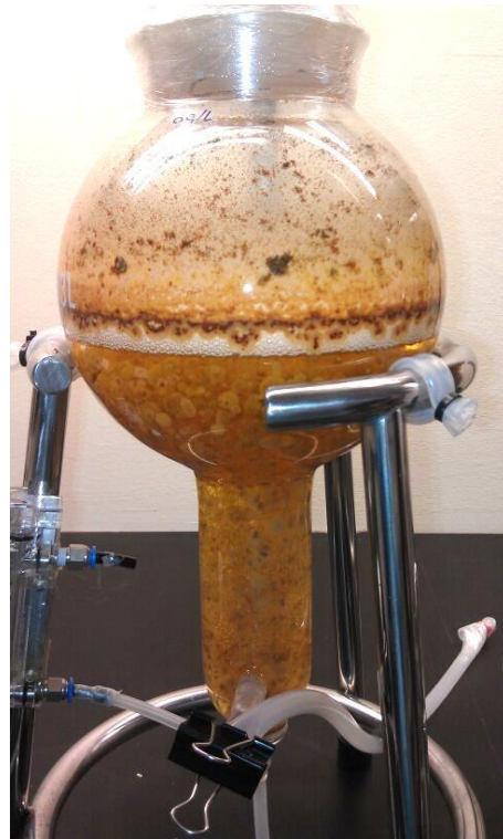
Figure 39: Contaminated air-lift bioreactor
