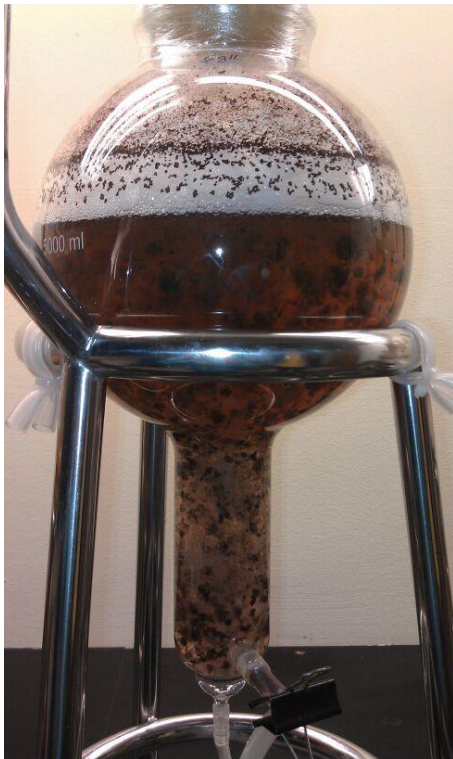
Figure 38: Air-lift bioreactor (6 g/L) after 1 week
