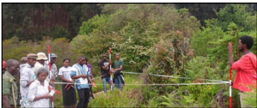
Survey team laying a quadrat using 3-4-5 method
