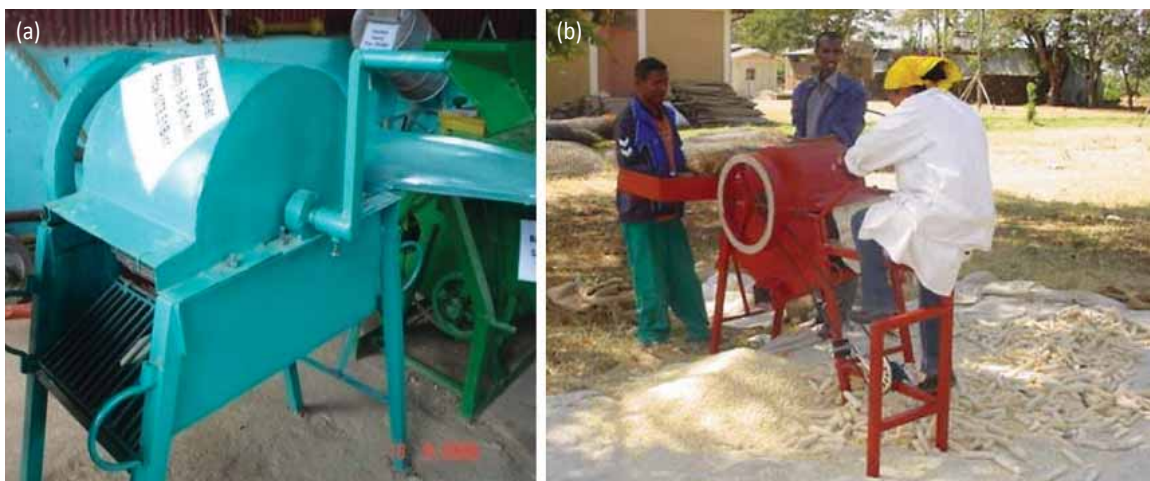
Figure 4. (a) Bako manual driven maize shellers (b) Melkasa Pedal driven maize sheller.
