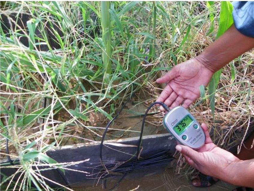
Photo B4: (Chapter 3) Competition trial with naked crabgrass and maize (grown to maturity) and the measurement of soil water content with a Decagon ECHO Check handheld meter.
