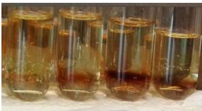
Figure A1.5 The brown ring at the interface of the two solvents is indicative of cardiac glycoside presence.
