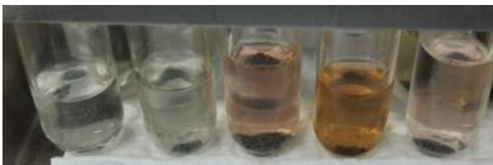
Figure A1.4 No flavanoids present in the two left samples but pink colouration indicates flavanoids in other 3 samples.
