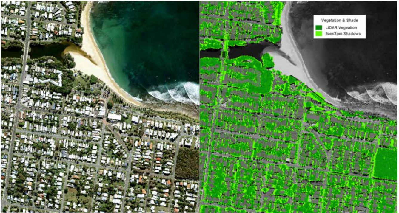
Figure 5: Shade is calculated using tree height and time of day within mapping software. The left image shows standard aerial photography, the right image, a LIDAR derived vegetation map with trees (non-ground vegetation) in dark green, and the 9am/3pm summer shadows in light green.
