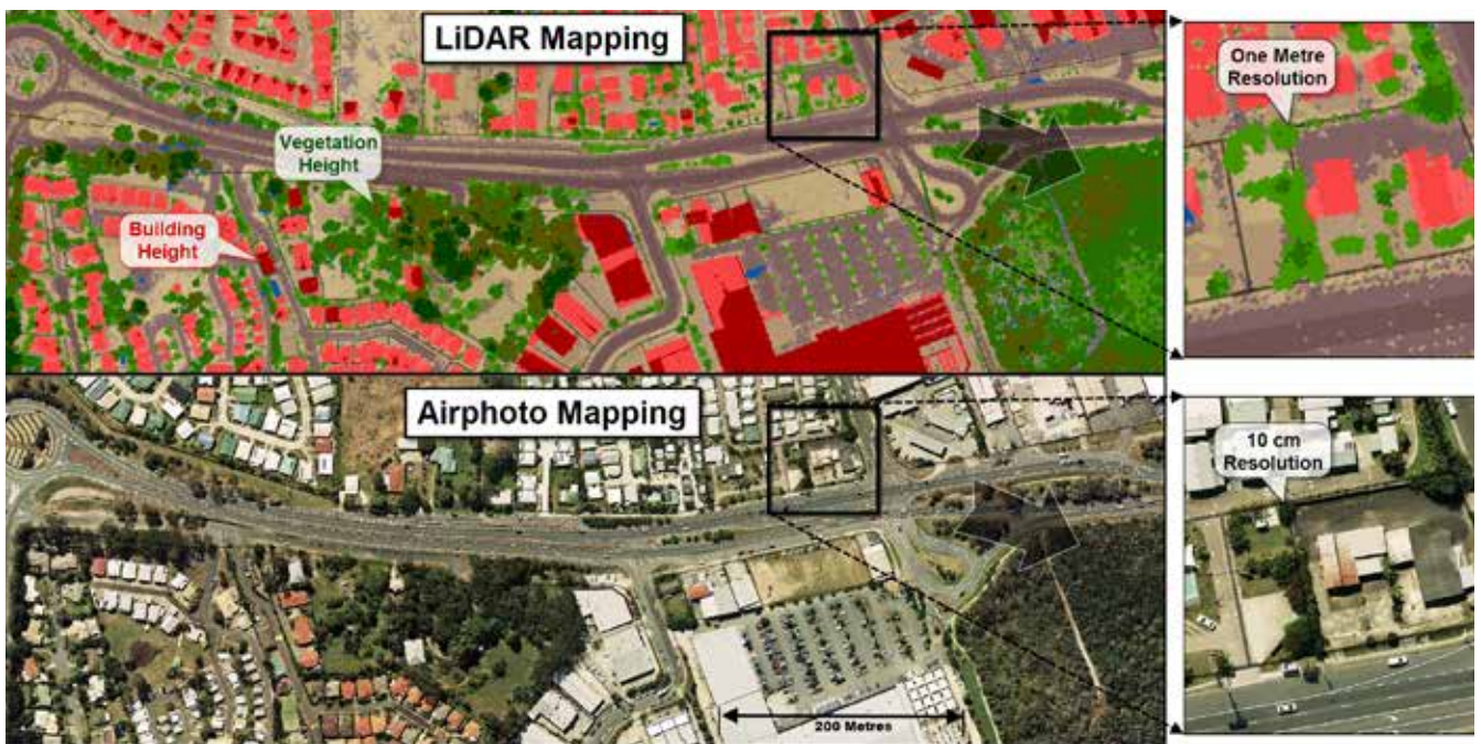
Figure 2: A comparison of standard aerial photography and LiDAR mapping. In the LiDAR mapping, buildings are represented by reds and pinks, vegetation in light and dark greens, and the ground in light browns and greys. The inset box (right side) shows the difference in mapping resolution when the view is zoomed in to a finer mapping scale. Whilst the LiDAR mapping has a lower one metre resolution, the vertical survey data can be exploited to automatically map many things, including topographic contours, building heights, and vegetation densities.
