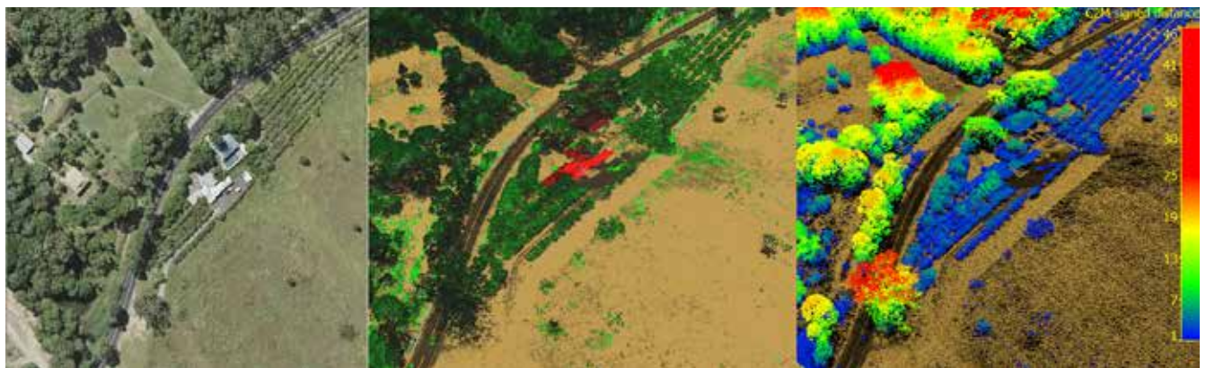
Figure 3: pictured from left to right: Aerial Orthophoto of a semi-rural area containing open grassed areas, regularly spaced fruit trees, a rural road and some natural vegetation; (MIDDLE) an oblique view of a coloured LiDAR data point cloud showing tree vegetation in green, buildings in red, and the ground in brown and black; and (RIGHT) the same LiDAR point cloud coloured according to height above ground in a range of colours from blue (shortest) through green, yellow and red (tallest).
