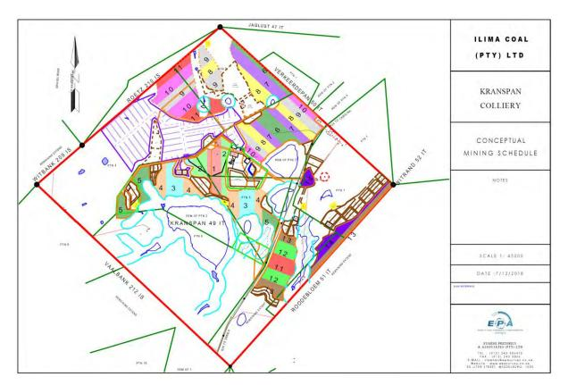
Figure 1. Plan showing opencast strip mine (shaded areas) with the planned mining per year sequence (Supplied by EPA).
