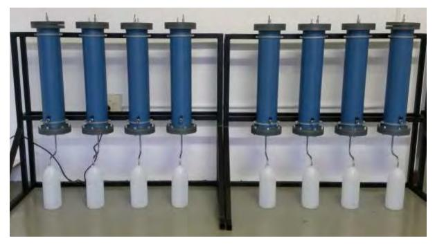
Figure 1: Photograph of the leach columns used to perform the kinetic tests
