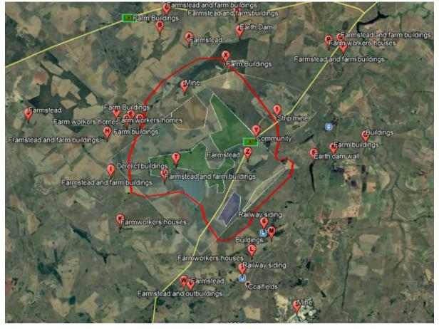
Figure 4. **Unmitigated** zone of influence for vibration >7.5 mm/s (area enclosed by the red line). Note the zones of influence will depend on where blasting takes place and the red line in this image represents the maximum zone of influence when mining reaches the boundaries. The shaded polygons represent the proposed opencast mine areas.
