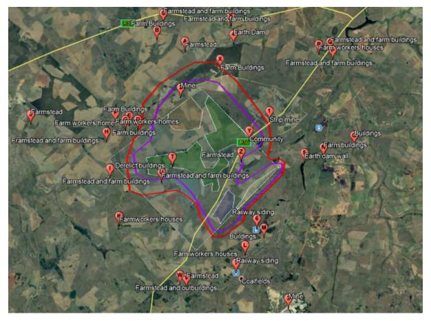
Figure 6. **Mitigated** zone of influence for vibration >7.5 mm/s (area enclosed by the purple line). The unmitigated zone of influence for >7.5 mm/s is shown for comparative purposes (red line). The shaded polygons represent the proposed opencast mine areas.
