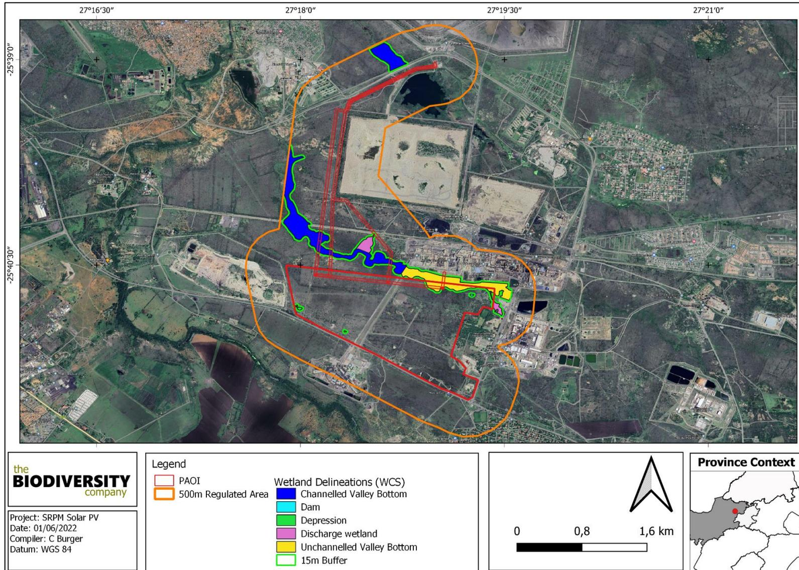
Figure 3-22 Recommended 15 m buffer zone for the delineated wetlands
