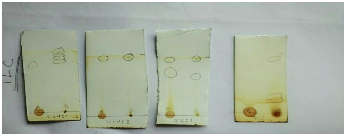
Figur-5: TLC with respect to Methanol extract of celosia cristata flowers Selected using different Mobile Phase solvent systems.
