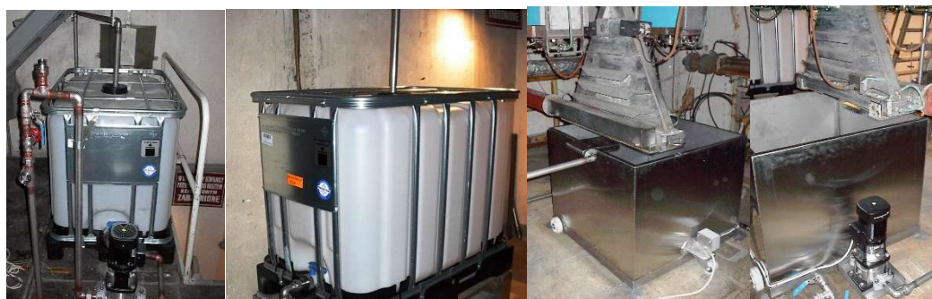
FIG. 10. Laboratory facility equipped with electron accelerator ILU 6 type: A) PP1 container, B) PP2 container, C, D) injection nozzle and stainless steel container (RV).
