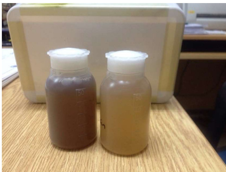
FIG. 2. Colour differences between pre-treated and npn-treated wastewater by ion exchange resin.
