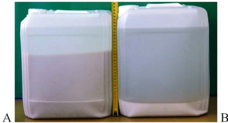
FIG. 6. Formation of layers upon sedimentation of raw industrial waste from brine purification and distillation stages. A) Brine purification products with calcium and magnesium ions, B) wastes from the production of soda.
