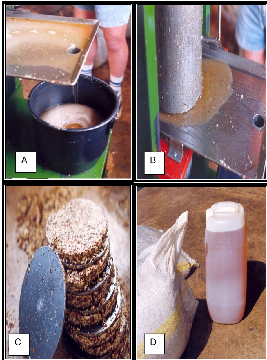
Figure 2.11 Oil processing machine (A); processed oil pouring into the container (B); seed cakes produced from pressed kernels (C) and twenty litre of processed marula oil (D).
