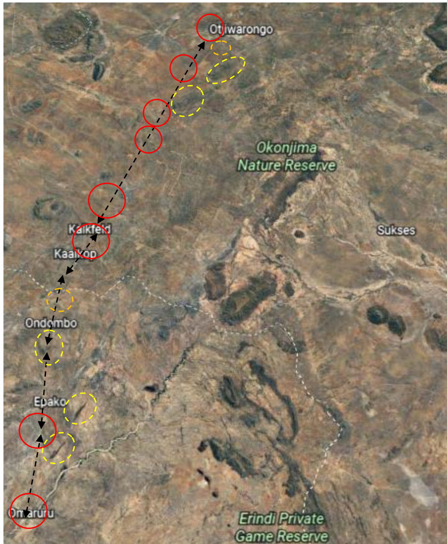
Figure 4. The approximate route of the Omaruru-Otjiwarongo rail link upgrades (black barred arrows). Red circles indicate ephemeral drainage line crossing points (e.g. Omaruru and Omatjene Rivers included); yellow oblongs indicate other important rocky areas (e.g. hills, ridges) and orange circles indicate ground dams.
