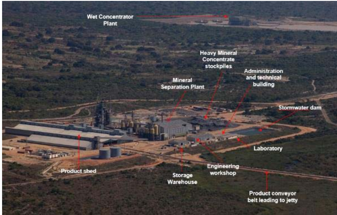
Plate 2.2: Aerial view of the existing Moma Mineral Sands project Mineral Separation Plant (MSP).
