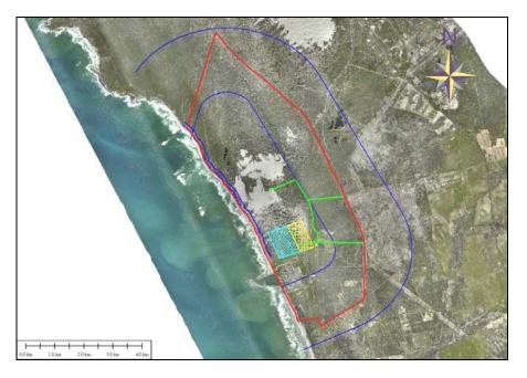
Figure 21: Recommended location for NPS (turquoise diagonal cross-hatching) and HV yard (yellow vertical cross-hatching) on the Duynefontein site (red outline). 800 m and 3000 m lines from EIA are shown in blue.
