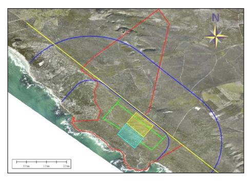
Figure 22: Recommended location for NPS (turquoise diagonal cross-hatching) and HV yard (yellow vertical cross-hatching) on the Bantamsklip site (red outline). 800 m and 3000 m lines from EIA are shown in blue.
