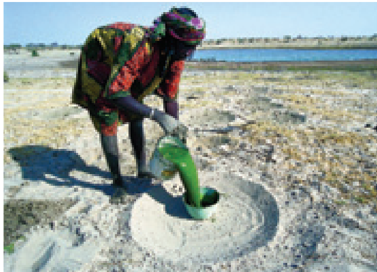
THE CONCENTRATED SOLUTION OF DIHÉ IS GENTLY POURED INTO A BOWL IN THE CENTRE OF THE SAND FILTER UNTIL IT OVERFLOWS
