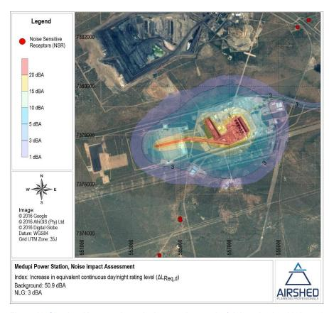
Figure 16: Simulated increase in equivalent continuous day/night rating level ( $\Delta L_{Req,dn}$ ) above the baseline
