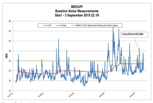
Figure 6: Baseline night-time noise measurement at noise sampling site 1
