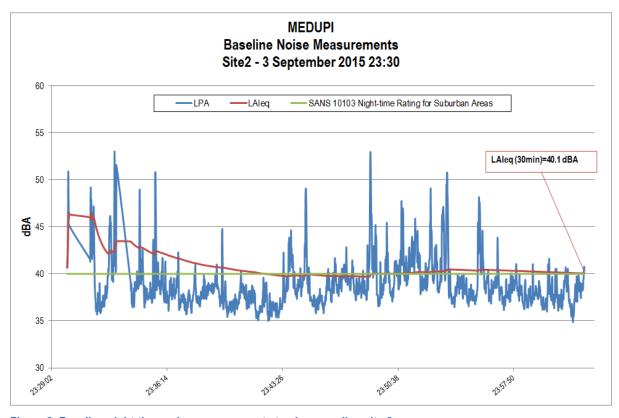
Figure 8: Baseline night-time noise measurement at noise sampling site 2
