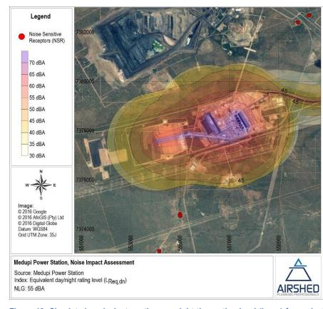
Figure 13: Simulated equivalent continuous night-time rating level ( $L_{\text{Req},n}$ ) for project activities
