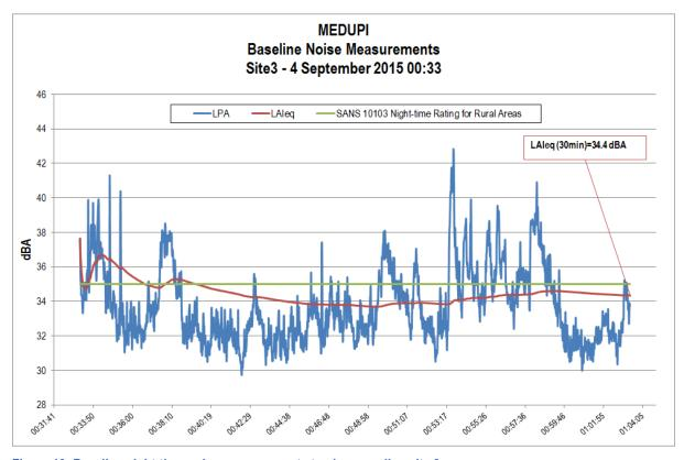
Figure 10: Baseline night-time noise measurement at noise sampling site 3
