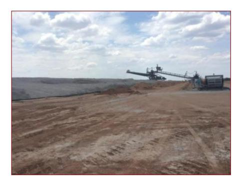
Figure 45- Machine that loads ash onto the facility from conveyor belt
