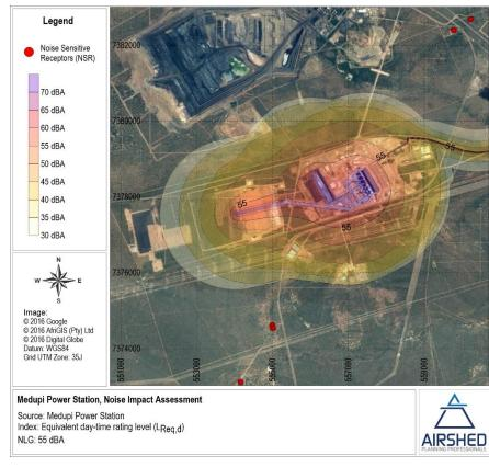
Figure 15: Simulated equivalent continuous day/night rating level (L<sub>Req,dn</sub>) for project activities
