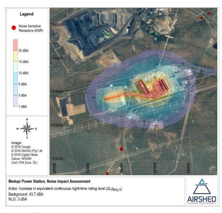
Figure 14: Simulated increase in equivalent continuous night-time rating level ( $\Delta L_{Req,n}$ ) above the baseline
