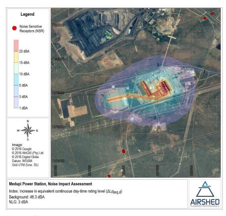
Figure 12: Simulated increase in equivalent continuous day-time rating level ( $\Delta L_{Req,d}$ ) above the baseline
