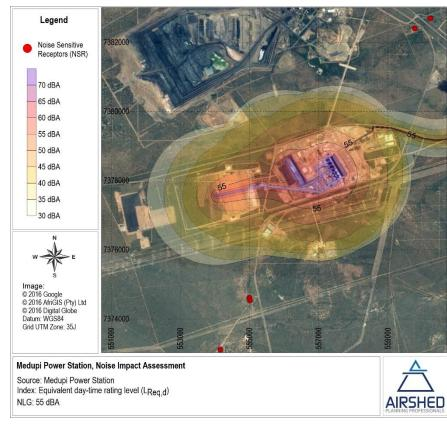
Figure 11: Simulated equivalent continuous day-time rating level (L<sub>Req,d</sub>) for project activities
