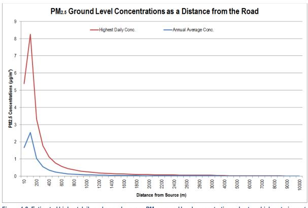
Figure 4-2: Estimated highest daily and annual average PM<sub>2.5</sub> ground level concentrations, due to vehicle entrainment, at set distances from the emission source
