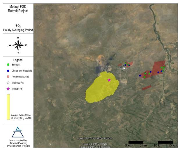
Figure 4-3: Area of exceedance of the hourly SO<sub>2</sub> NAAQS due to Matimba Power Station operations and Medupi with FGD
