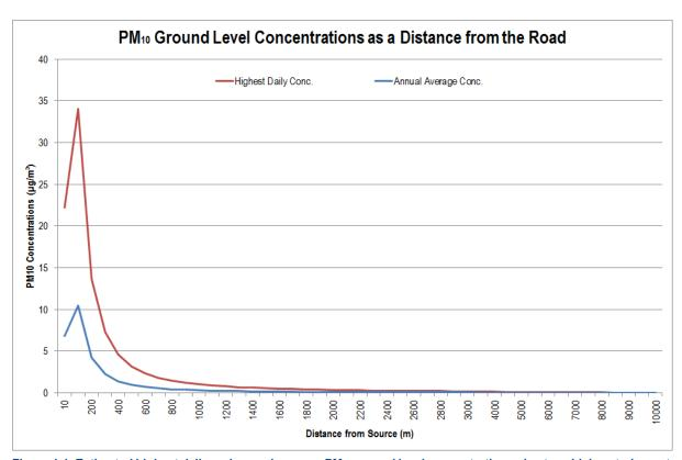
Figure 4-1: Estimated highest daily and annual average PM<sub>10</sub> ground level concentrations, due to vehicle entrainment, at set distances from the emission source
