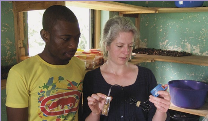
Testing the relative humidity of seeds using a TinyTag Data logger, Plant Genetic Resources Research Institute, Ghana PHOTO: TIM PEARCE
