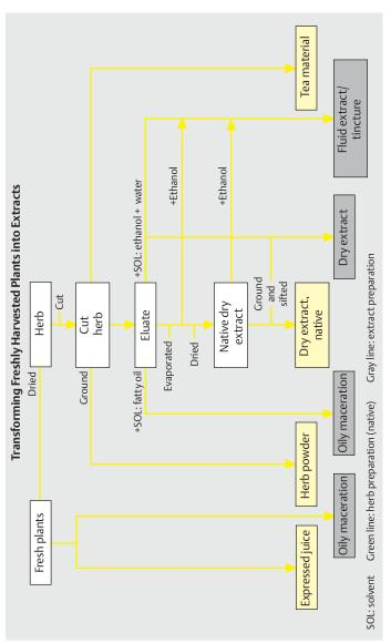
Fig. 1 The process of manufacturing plant extracts.
