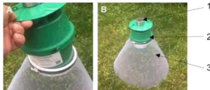
**Figure 2.** Details of the sweetpotato weevil trap to use in the MAT. The base of the trap is a funnel made with galvanized mesh (3). This allows weevils to walk to the bucket trap fitted within a PVC ring that holds the funnel (2). The bucket trap includes a solar cell (1) that charges an LED diode
