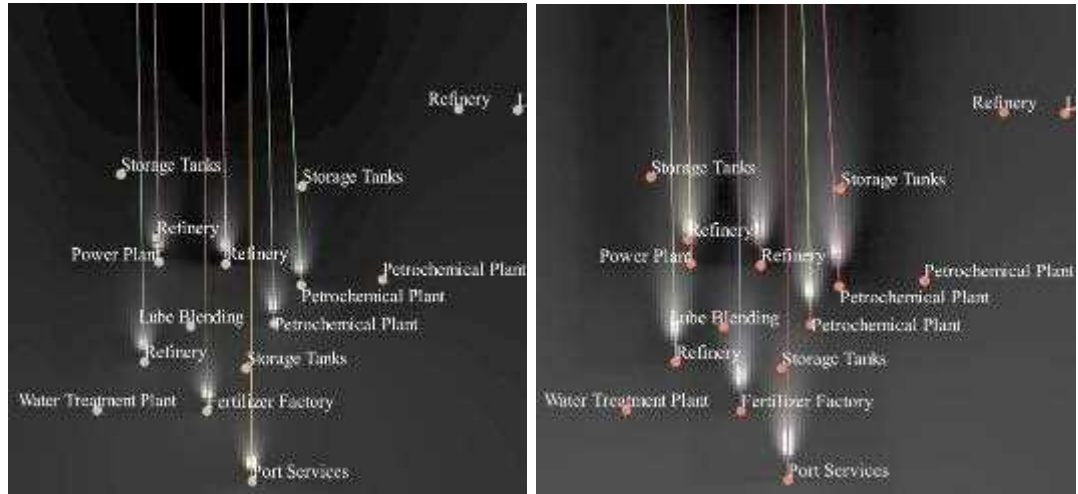
Figure 5.15: Cumulative impact of Gaussian Plume Model output of all the seven stack emissions under a: Class A and b: Class B of Pasquill atmospheric classes of weather condition
